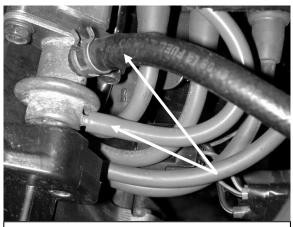
**c)** Remove the fuel return line and vacuum line from the fuel pressure regulator.
