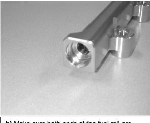
**b)** Make sure both ends of the fuel rail are clean and free of debris and burrs.
