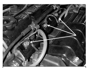
**d)** Remove the three fuel rail mounting bolts. The two outer bolts have throttle cable mounting brackets on them. Removing the throttle cable from the brackets and tucking it out of the way before removing the bolts may simplify removal/installation of the fuel rail.
