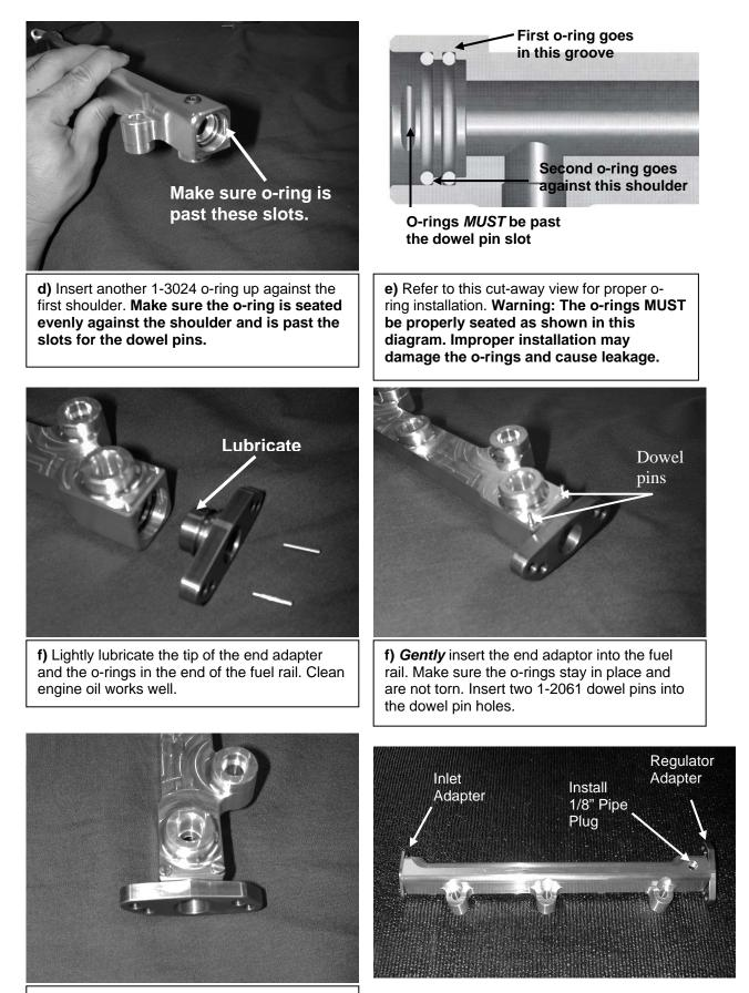
**g)** Insert and tighten two 1-2062 screws into the dowel pin holes. Repeat steps b-g for the other side of the fuel rail.
