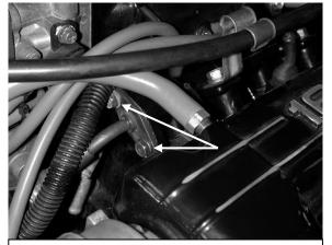
**a)** Remove the two bolts mounting the highpressure fuel inlet line to the fuel rail. Wrap a rag around the fitting and pull it clear of the fuel rail.
