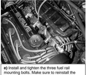
e) Install and tighten the three fuel rail mounting bolts. Make sure to reinstall the two throttle cable brackets on the outer fuel rail bolts.
